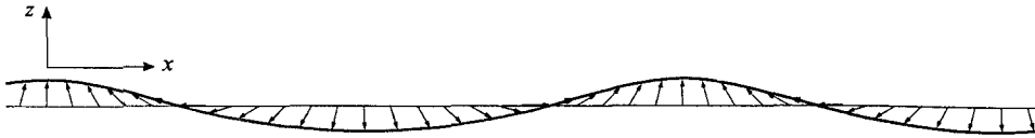
FIGURE 1. Sketch of an initially horizontal material contour and the associated displacement field \xi(\mathbf{x}, t) in a deep-water wave, for one value of z and a number of equally spaced values of x . The horizontal line marks the given value of z . By (6), the latter gives the mean depth of the set of material particles located at the tips of the displacement arrows (i.e. at positions \mathbf{x} + \xi ). Note that, because the average is evenly weighted over x rather than x + \xi , the horizontal line lies higher than a line cutting off equal areas.
